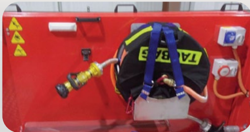
Hose Reel on Platform (electric rewind)
